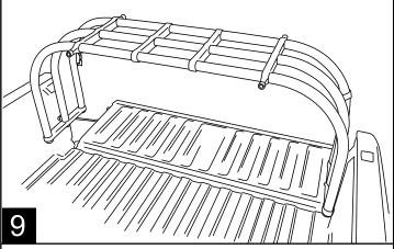
Adjust bumper uprights so that the rubber bumper rests on a flat surface on the tailgate.
