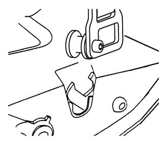
When the Bed Extender is at the furthest rear position, push down on the buckle to insert into tailgate latch. Tighten straps. To release, pull tailgate handle.
