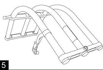
Secure pivot upright with large wedge and PT screw. Torque to 20 in. lbs.
