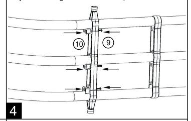
Place assembly on flat surface as shown. The tube ends should extend through the pivot upright approximately. 3/8"
