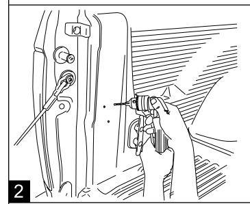
Using a power drill and 9/64" drill bit, drill through the sheet metal. If equipped with a bedliner, drill through bedliner.
