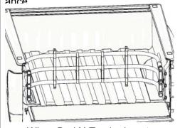
When Bed X-Tender is out on the tailgate be sure to fasten strap latches properly.
