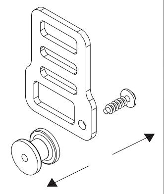
Install 1 piece insert with the provided 10/32 x 7mm socket head cap screw with a 4mm hex key. Repeat for other strap.
