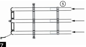
Adjust the width of the Bed X-Tender by placing the pivots into the mounting brackets.
