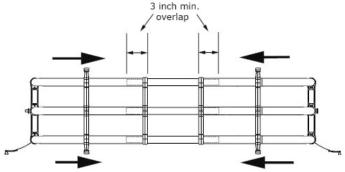
\*For flareside trucks using compact Bed X-Tender cut 4" off of each half of bent tubes.
