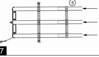
Connect the two halves. Make sure there is at least 3" overlap with the bent tubes on each side.
