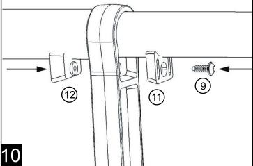
Rotate Bed X-Tender into the bed and check that the rubber bumper position is on a flat surface. Torque PT screws to 20 in. lbs. Close tailgate and check for clearance
