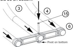
Insert Phillips screw through pivot upright and predrilled center tube. Torque screw to 18 in. lbs. Slide strap latch over outside tube with plastic insert facing up. (Passenger side shown, Driver side opposite.)
